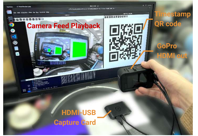
Fig. A1: Camera Latency Measurement
