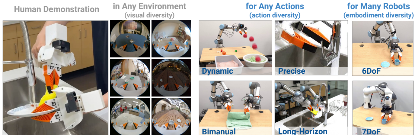
Fig. 1: Universal Manipulation Interface (UMI) is a portable, intuitive, low-cost data collection and policy learning framework. This framework allows us to transfer diverse human demonstrations to effective visuomotor policies. We showcase the framework for tasks that would be difficult with traditional teleoperation, such as dynamic, precise, bimanual and long-horizon tasks.
